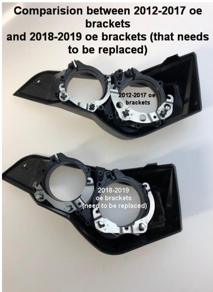
See comparison picture below between the 2012-2017 oe aluminium brackets and the replacement brackets from RJWC. The RJWC brackets don't have the pressed pattern on the brackets (see adjustment info below) . Below is the correct installation and alignment.
