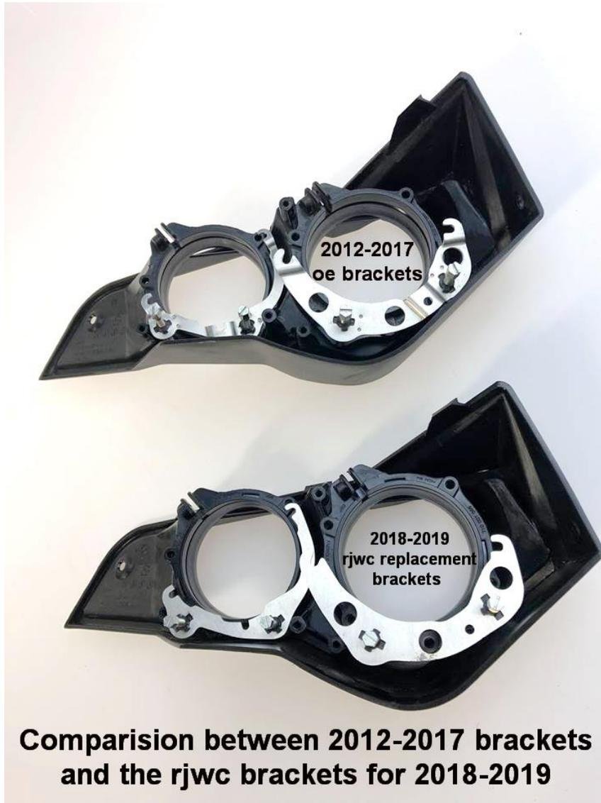
Below is instructions on how you loosen and tighten the plastic tabs that holds the alloy brackets in place. Use a plier to turn them into position and also use the plier to keep them in place while adjusting.
