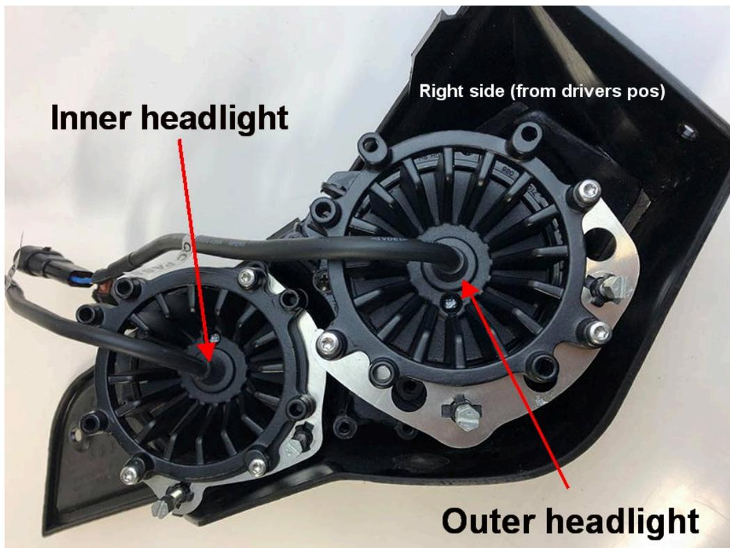
Use a 4 mm allen key (or similar) while doing the adjustments on the RJWC replacement brackets so that the plastic tabs don't slide out of position
